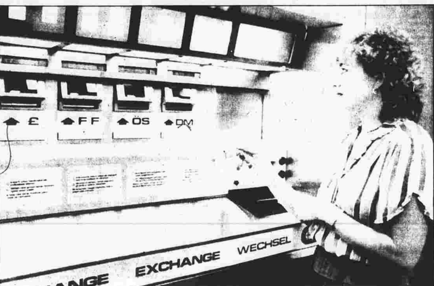
A customer demonstrates an automatic foreign-exchange machine at the Union Bank of Switzerland in Zurich. The electronic machine, which opened for use in 1985, is able to change German, Austrian, French and British banknotes into Swiss francs.
